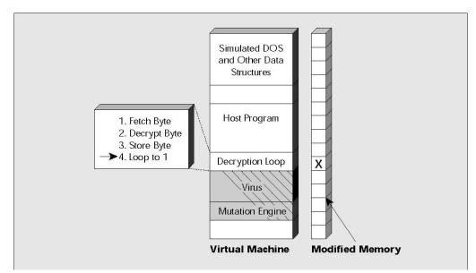
**Figure 7.** At this point the generic decryption engine passes control of the virtual machine to the virus and the virus begins to execute a simple decryption routine. As the virus decrypts itself, the modified memory table is updated to reflect the changes to virtual memory
