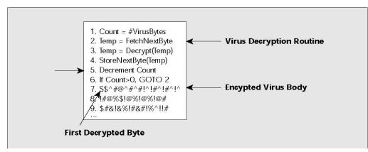
Figure 3. At this point, the virus has executed its first five instructions and has decrypted the first byte of the encrypted virus body
